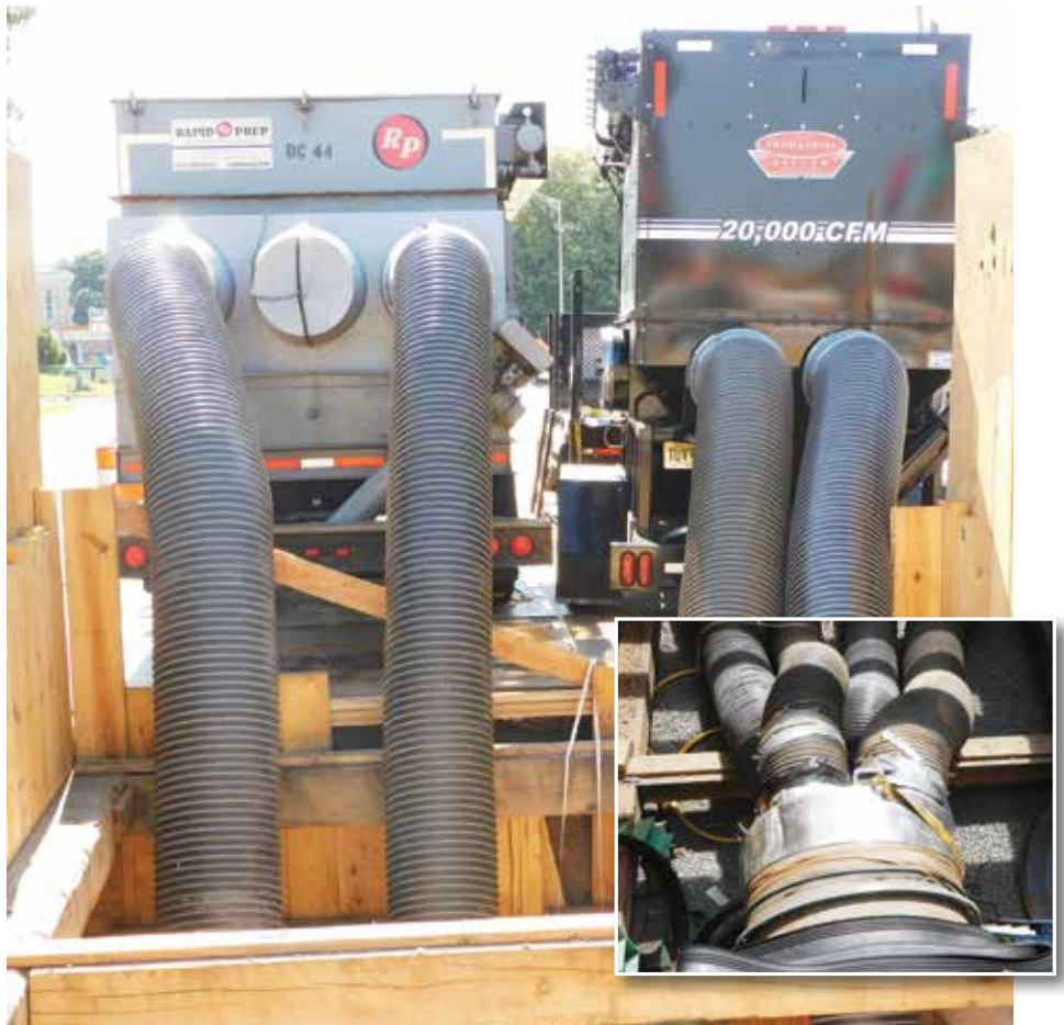
Maintaining a minimum 45mph velocity was an achievement, considering pipe diameter and geometry
