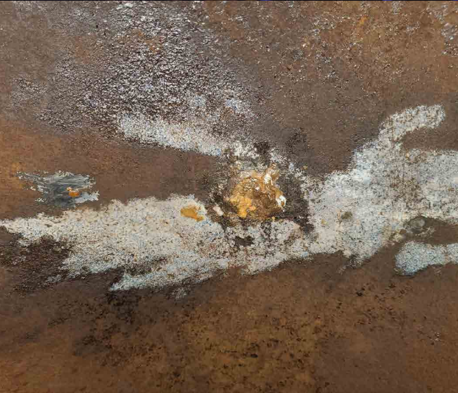
Corroded 30x36 in (760x910 mm) diameter steel reducer.
