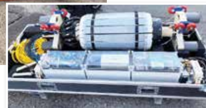
Figure 1. A pig-like tool covered with sensors is tethered through the main
