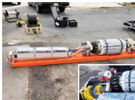
Figure 1. A pig-like tool covered with sensors is tethered through the main
