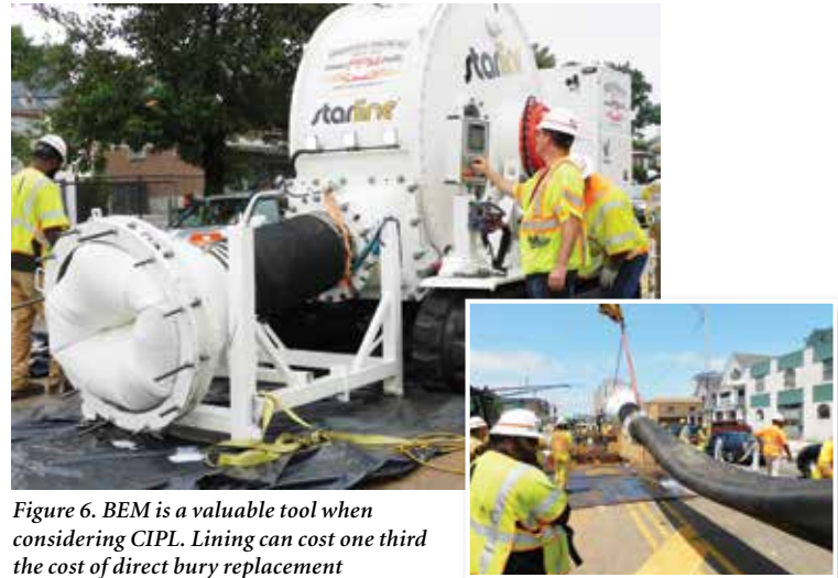
Figure 5. Sensor blanket for BEM external Flexible Array Scanning Tool (FAST) wraps around the pipe
